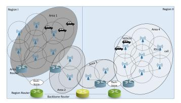
Fig. 2. Example Vehicular Network Topology
