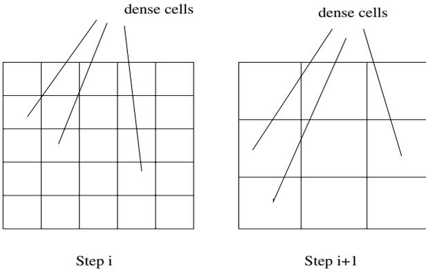
**Fig. 4.** At step  $i$ , a set of grid cells (in the 5-regular grid in this example) are selected to be added in the GENHIST estimator. At step  $i + 1$ , a new set of cells, from a coarser grid (3-regular in this example) are selected to be added in the GENHIST estimator. Buckets from different grids can overlap
