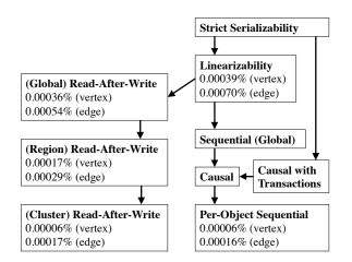
Figure 8: Spectrum of consistency models with arrows from stronger to weaker models. Measured anomaly rates are shown. Bounds on the anomaly rate in unmeasureable non-local consistency models can be inferred.
