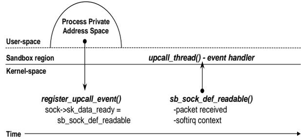
Figure 3. Event handling control flow.
