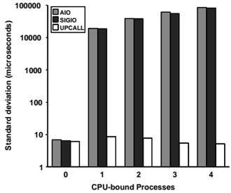
**Figure 6. UDP message transmission jitter.**
