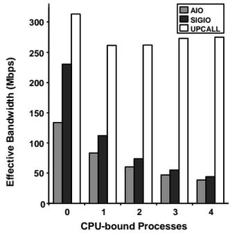
Figure 4. Effective bandwidth achieved in UDP stream transmission.
