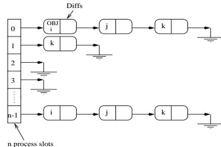
Figure 2: A sample slotted-buffer at local process 2. There is nothing to send to process 3.
