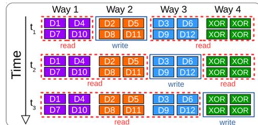
Fig. 4: The set of write flash chips rotates to a different way after a block of data is written to each write flash chip.
