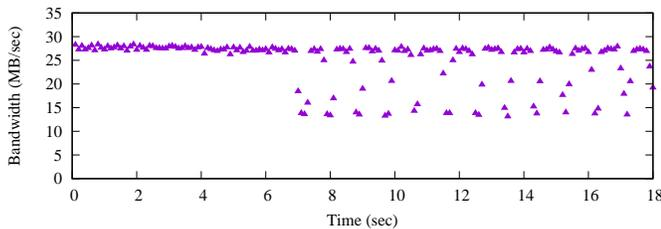
Fig. 16: The effects of garbage collection on write bandwidth with WAO-GC. Garbage collection is initialized after 7 seconds.
