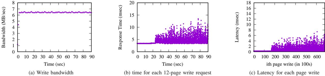
Fig. 11: Write bandwidth, request response time, and page latency with WAO-GC FTL.
