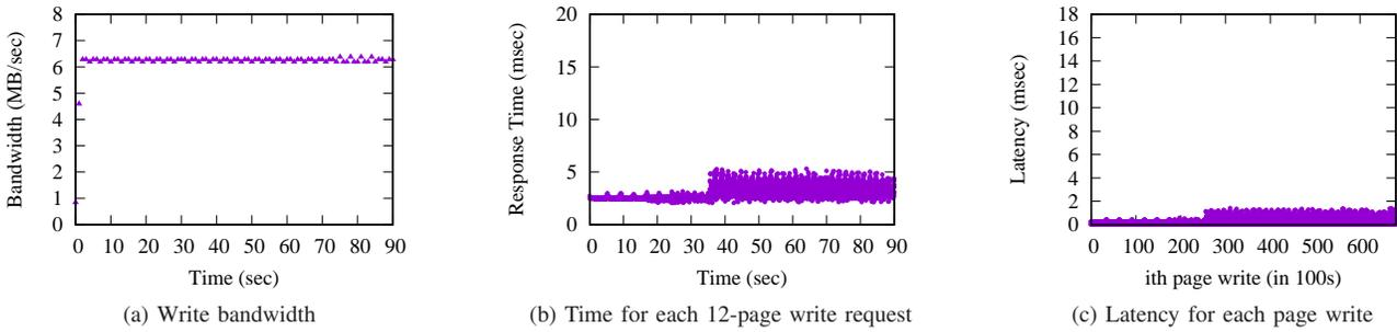
Fig. 10: Write bandwidth, request response time, and page latency with PaRT-FTL.
