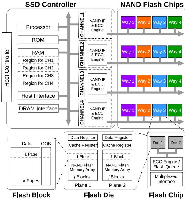
Fig. 1: SSD internal architecture.
