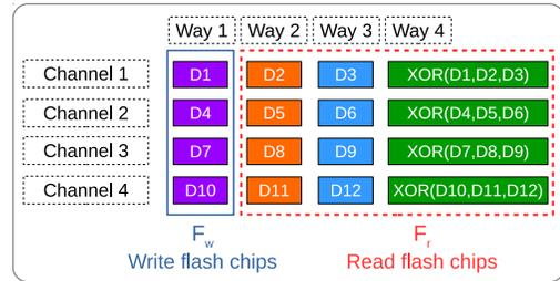
Fig. 3: Flash chip layout. In this example, there are 12 flash chips storing data and 4 flash chips storing encoding pages. Flash chips being written to are on Way 1 of each channel, while other flash chips are servicing read requests.
