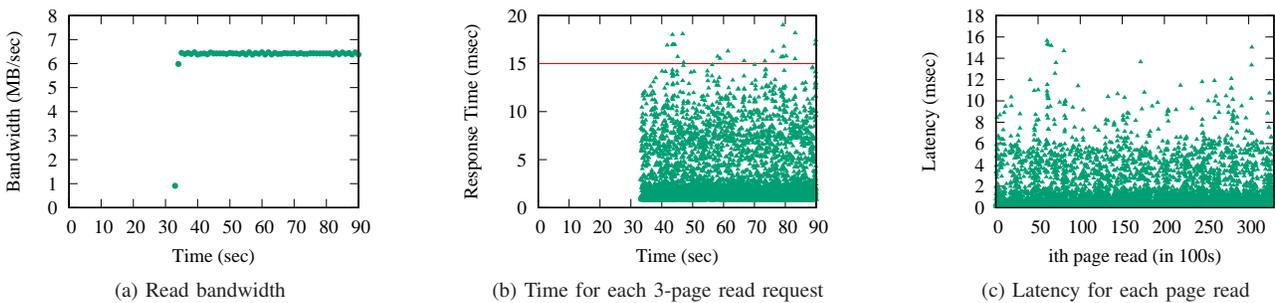
Fig. 13: Read bandwidth, request response time, and page latency with WAO-GC FTL.
