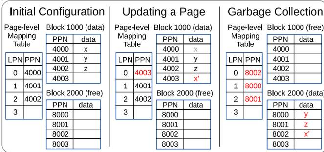
Fig. 2: Page-level mapping and block reclamation. Every logical page number (LPN) is mapped to a physical page number (PPN). When overwriting LPN=0, the updated data  $x'$  will be written to a different physical page since in-place updates cannot be performed; the mapping is updated accordingly. When the SSD fills up, garbage collection is triggered and valid pages in a victim block are copied to a free block and the victim block is erased.
