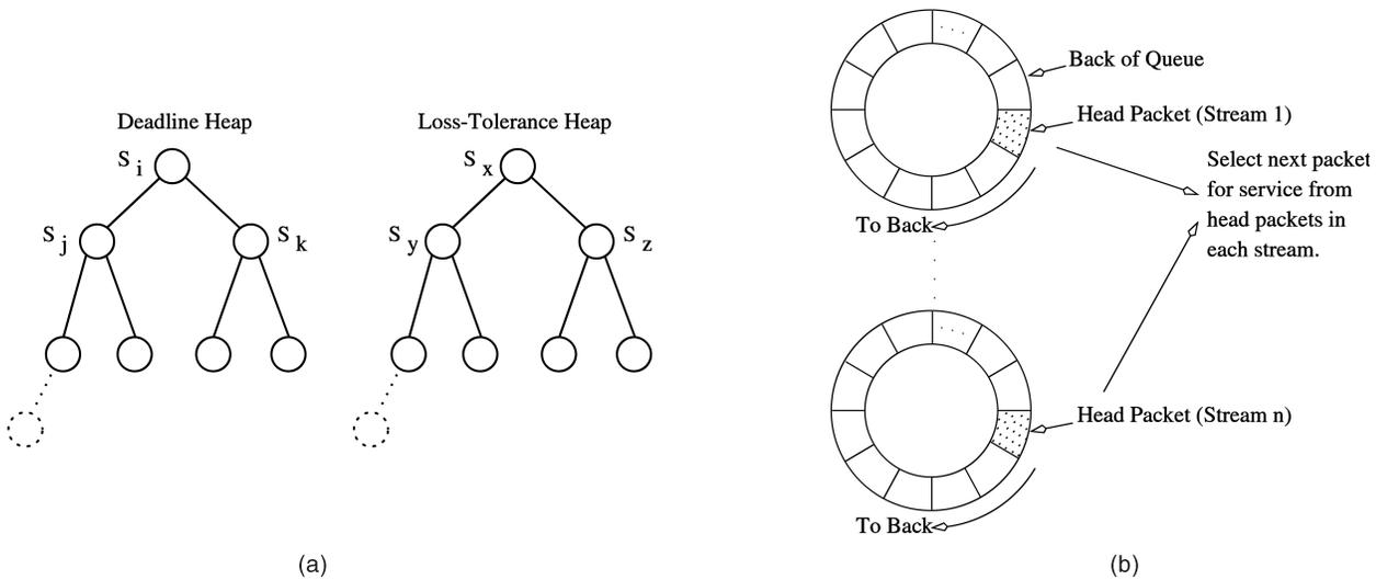
Fig. 3. (a) The NI implementation of DWCS uses two heaps: one for deadlines and another for loss-tolerances. (b) Using a circular queue for each stream eliminates the need for synchronization between the scheduler that selects the next packet for service and the server that queues packets to be scheduled.
