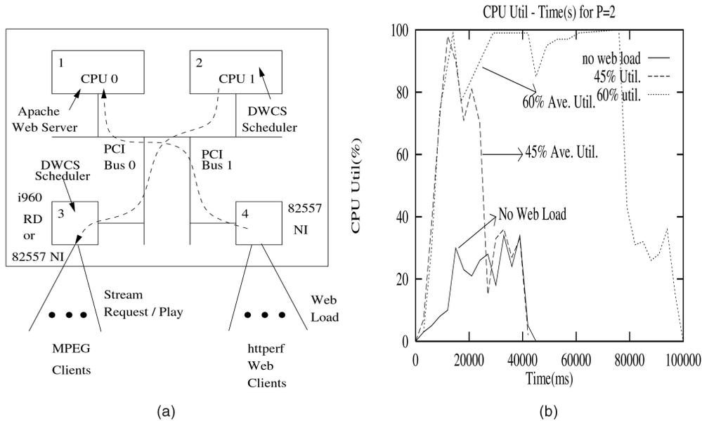
Fig. 4. (a) Server loading architecture—Web and media traffic. (b) CPU utilization variation with server load.
