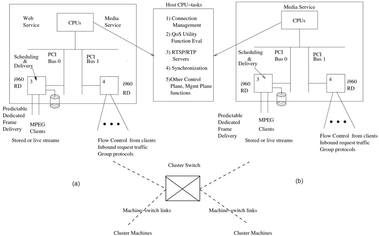
Fig. 1. Cluster hardware: Host CPU, NI CoProcessor, and interconnect. (a) Multiservice servers and (b) single-service servers.
