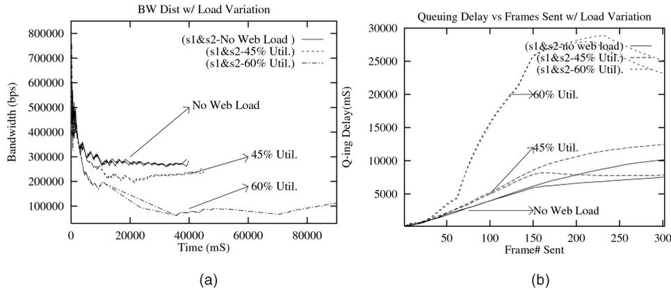
Fig. 5. (a) Bandwidth variation with load. (b) Queuing delay variation with load.
