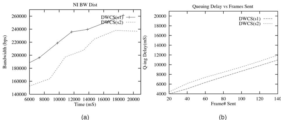
Fig. 6. (a) NI Bandwidth distribution snapshot: unaffected by system load. (b) NI Queuing delay snapshot: unaffected by system load.
