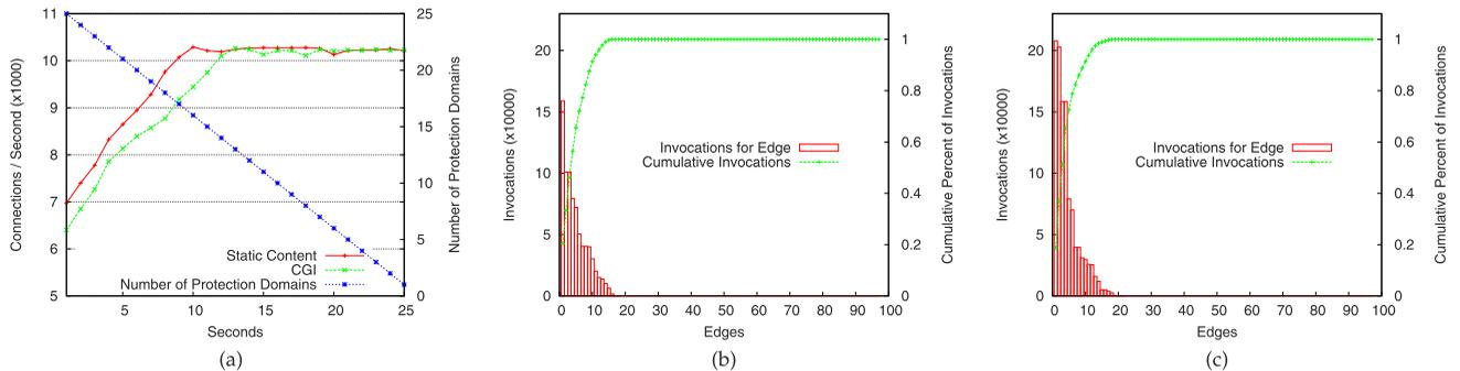
Fig. 5. (a) The effect on throughput of removing protection domains. (b) and (c) The number of invocations between components, and the CDF of the invocations for (b) HTTP 1.0 static content requests, (c) persistent HTTP 1.1 CGI requests.
