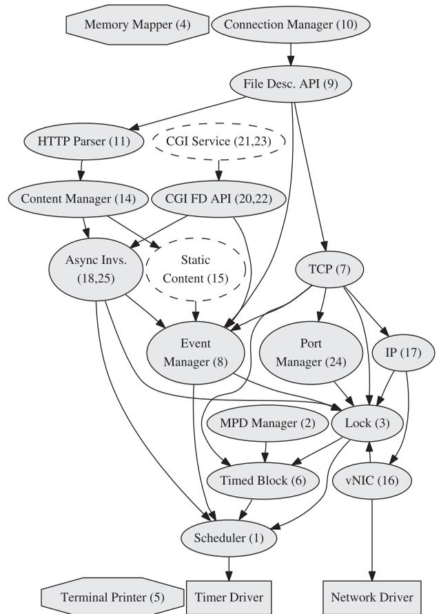
Fig. 3. COMPOSITE component-based webserver.
