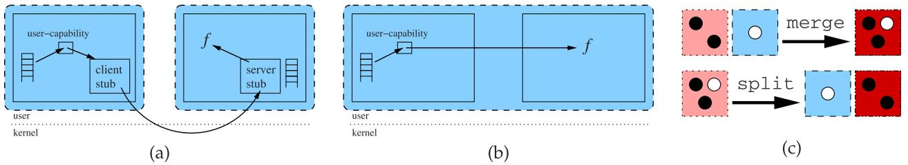
Fig. 1. (a) and (b) Invocation methods between components (solid boxes). (a) Invocations between protection domains (shaded, dashed boxes). (b) Intraprotection domain invocations. (c) MPD primitive operations.
