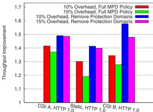
Fig. 6. The throughput improvement over full isolation.
